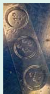
Making the vacuum formed chocolate moulds
