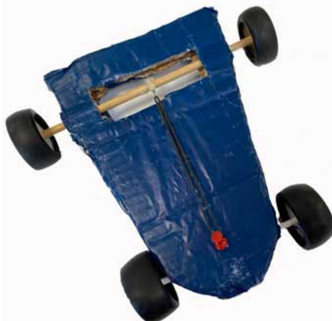
A model to show how elastic potential energy can be used to produce kinetic energy.
